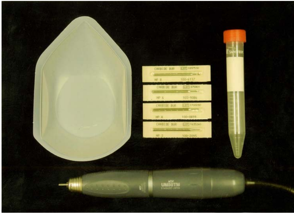
FIG. 1—Armamentarium including a weigh boat, long-shanked round burs, 15 mL polypropylene reagent tubes, and laboratory handpiece.
